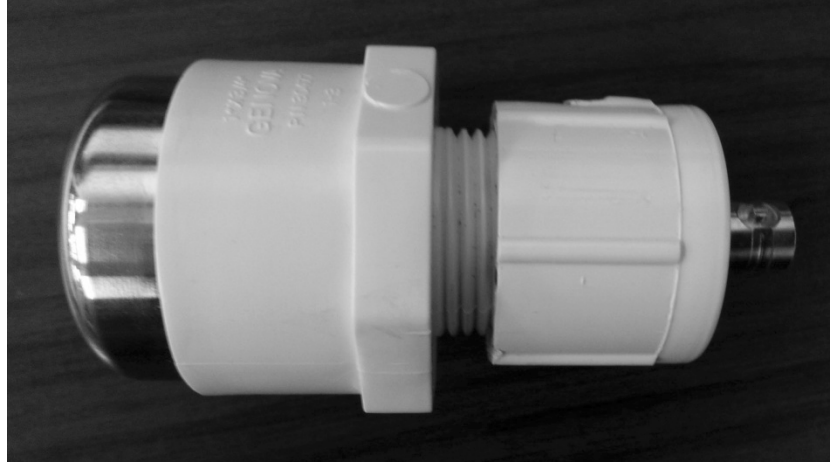
Figure 2.3 – Ultrasound Transducer with a stainless steel housing and PVC handle
